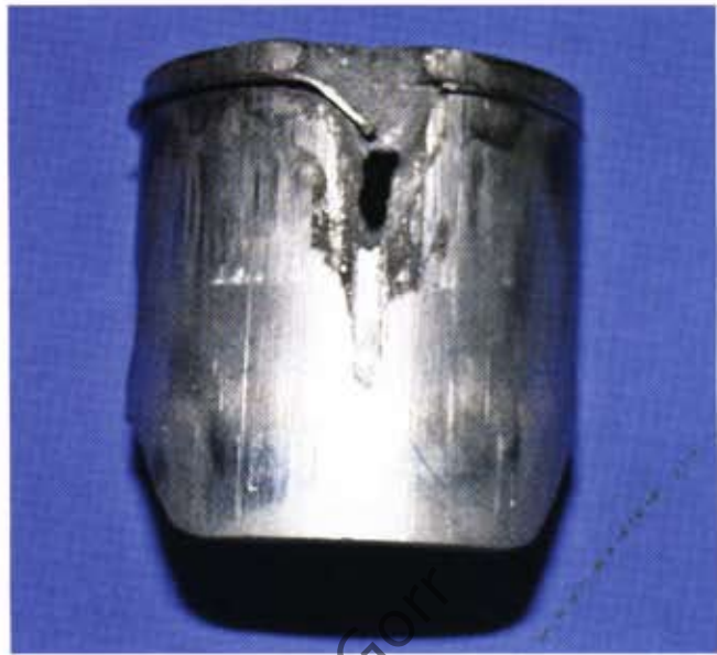
This piston has a hole burned on the exhaust side. The engine had a blown left crankshaft seal and an air leak that leaned the carb jetting.
