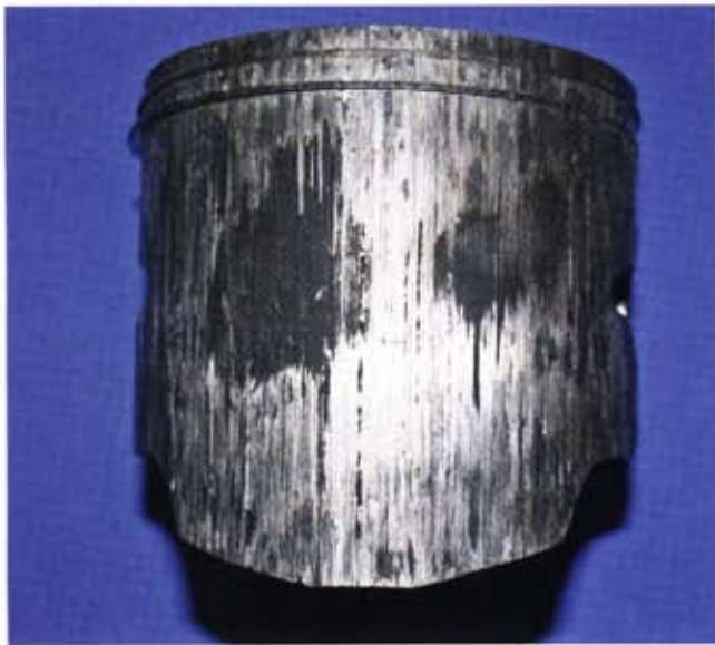
This piston is deeply scratched and dry because the engine was run with straight gas and no premix oil.
