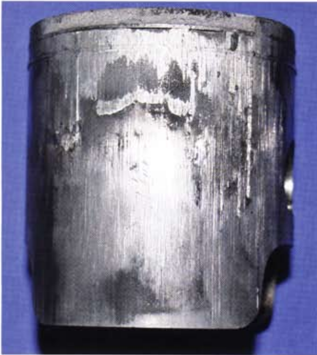
This piston overheated from a blown head gasket that forced all the coolant out of the blow-off vent hose.
